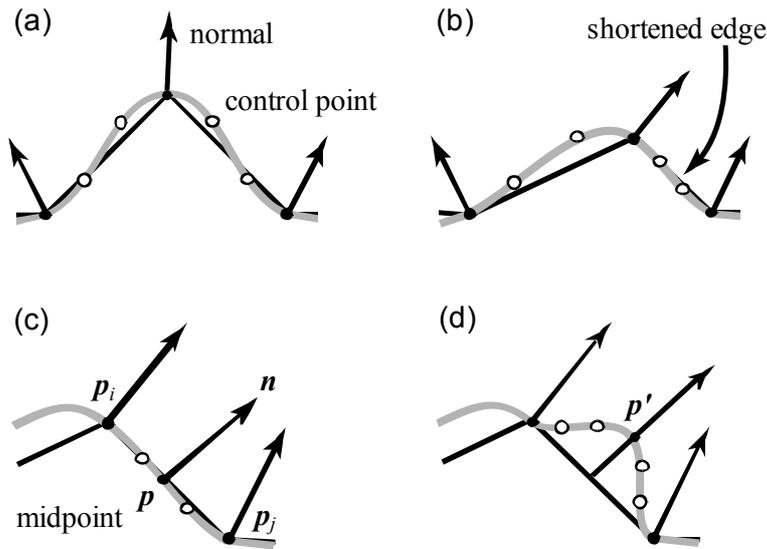
Figure 4.5 Edge length control in section view. (a) Original edges in the at rest length. (b) When an edge is shortened, (c) the midpoint of the shorter curve is controlled (d) so that the curve length is close to the original edge length.
