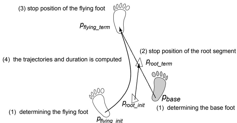
Figure 3.5: Motion planning for protective step.
