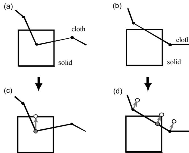
Figure 4.6 Collision detection and penetration avoidance. (a) Cloth vertex and solid penetration. (b) Cloth face and solid intersection. (c) Cloth particle or (d) cloth face position is corrected and constrained.
