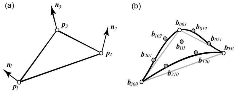
Figure 4.2 PN triangles replace a triangular face by a three-sided cubic Bezier patch computed from the three positions and normals. The cubic Bezier patch is represented by coefficients or control points ( $B_{ijk}$ ).
