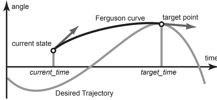
Figure 2.4 Tracking control using Ferguson curve.
