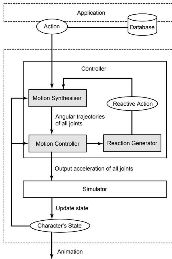
Figure 3.1 System structure.
