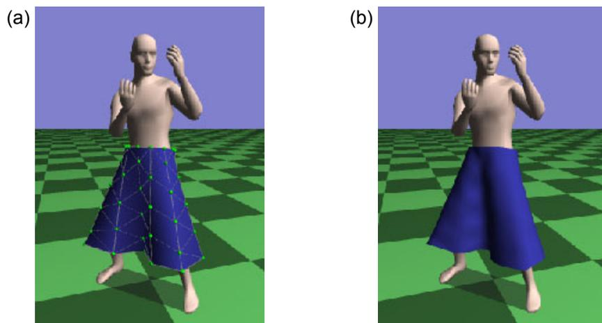
Figure 4.1 An example of the proposed approach. (a) A small number of particles (66 particles in this case) are controlled using dynamic simulation. (b) The cloth surface is then smoothed using geometrical techniques (1,944 faces were rendered).
