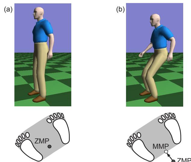
Figure 2.3 Zero-Moment Point in (a) balanced and (b) unbalanced state.
