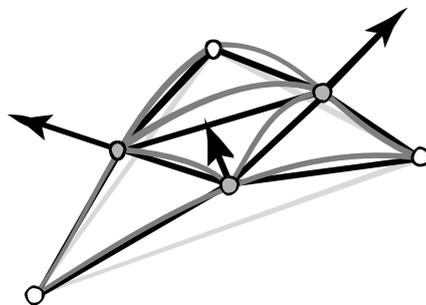
Figure 4.4 A cubic Bézier patch (Figure 2(b)) divided into 4 cubic Bézier patches. The 3 midpoints are obtained from the original PN triangle.
