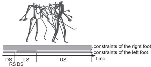
**Figure 2:** Example of the support phases and constraints between the feet and ground. In this kick motion, after the left foot is slightly moved (RS), the right foot is moved (LS) and then both feet touch the ground (DS).
