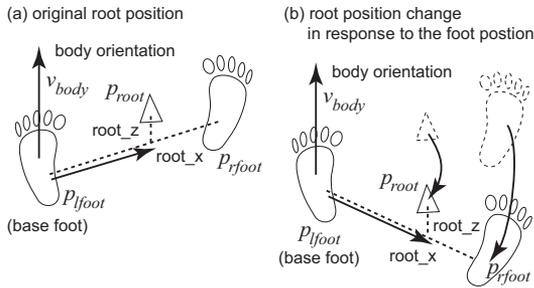
**Figure 9:** Transformation of the horizontal position of the root (pelvis) in response to the changes in foot positions.
