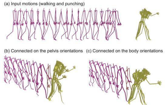
**Figure 8:** Example of body orientations and motion connection based on them. If two motions are connected based on the pelvis directions (b), the following motion goes into wrong direction. This is solved by using body orientations that are computed from the movement of the pelvis (c).
