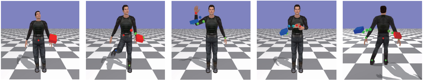
Figure 5: Images from a demonstration of our interface. Inputs from the hand motion sensing device are visualized on the screen. The rectangles represent the user’s hands (red: right hand, blue: left hand). The spheres represent the user’s fingertips (green: finger bent, red or blue: finger extended). The spheres on the character are controlled points (red: controlled by right hand or fingers, blue: controlled by left hand or fingers, green: not controlled, but the corresponding finger is recognized).
